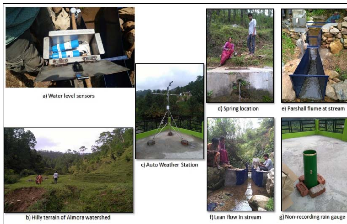
Figure 4: Instruments installed in the watershed of Almora
