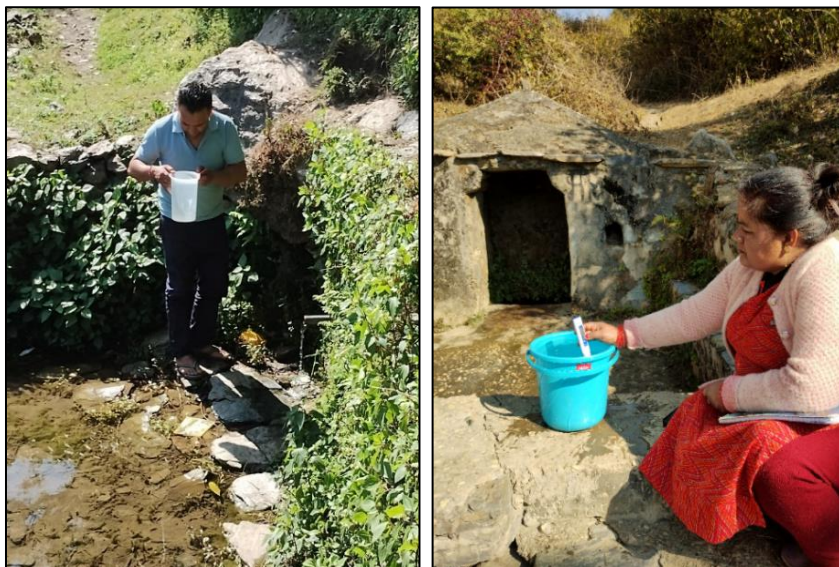
Para-workers recording discharge and in-situ water quality
